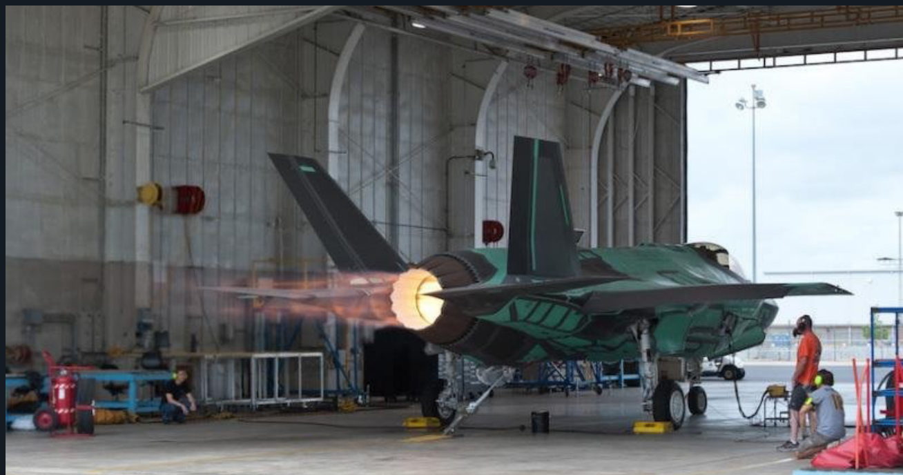
Engine Warm Up is possible inside the hangar with ILDFA
